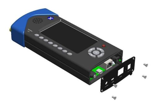
Remove and replace the LAN end plate.
