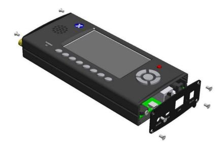
Each case half contains a printed circuit board connected via 2 multi-way connectors located under the row of switches. When separating the case, gently pull the 2 halves apart without twisting as this may cause damage. There is also a speaker cable linking the case halves in the SxA and fan and speaker cables in the SxD and SxE.
