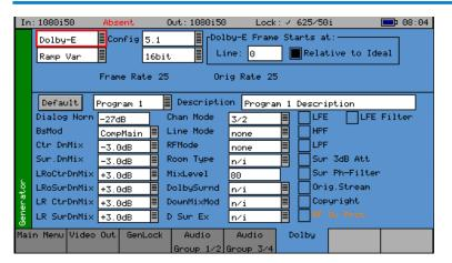
The Sx instrument Dolby Generator software option allows generation of Dolby-E, Dolby Digital and Dolby Digital Plus pre-encoded test signals to check that they are transferred transparently through the broadcast chain unaffected by routers/switchers, satellite links, etc.
