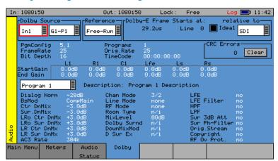
This displays the Program configuration (5.1 + 2 etc), the number of program in the meta-data, the frame rates and bit depths and time-code if any present.
