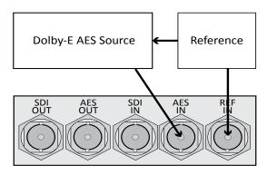
In the example above, the AES signal contains a Dolby-E stream. The Sx instrument needs to lock its internal audio clock to the external reference signal (Generator – Genlock – Source = 1 Ref) and the Dolby Timing source should be set to Ext.Ref. The AES source MUST be locked to the same reference as the Sx.
