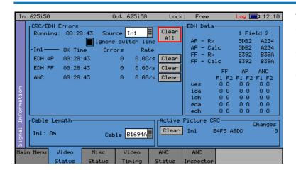
The Video Status menu display the status of the selected video input and displays any errors that have been found in the data stream.
