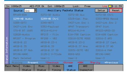
The ANC status menu shows which ANC packets are present on the SDI input and whether they have any errors. Each field is colour coded according to whether the ANC packet is present (White), missing (Grey), has errors (Red), or has previously had errors (yellow).
