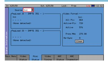
The Misc Status menu display the status the SMPTE 352 packets embedded in the selected video input and displays any errors that have been found.
