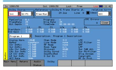
The Dolby-E status option allows display of the Dolby-E meta-data present in the selected audio stream and determines whether the Dolby-E packet is timed correctly on the SDI video stream.
