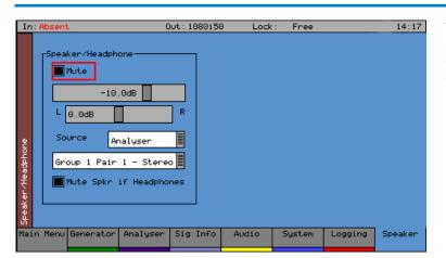
The Speaker menu controls which audio pair that can be heard on the loud speakers and headphone output of the Sx instrument.
