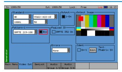
The Sx instrument can create video test signals for all supported SD and HD SDI output standards including the 3GHz standards at 1080p/50/59/60. It will support Y,Cr,Cb formats as well as RGB formats.
