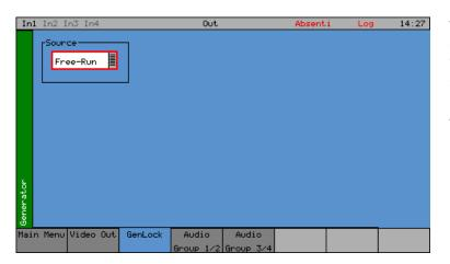
The Sx instrument can create video test signals that are either free-running or locked to a studio reference signal.
