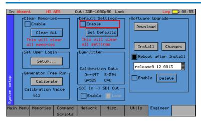
The Engineer menu is used to manage the Sx instrument and allows user access to be setup and the installation of new versions of software.
