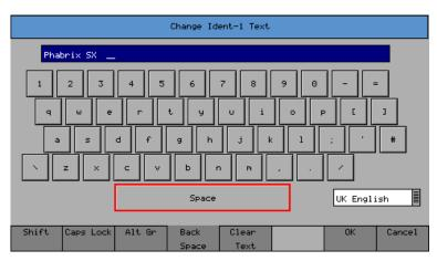
When editing text, the keyboard above is displayed to allow easy editing. Move the cursor to select the key to 'press' and then press 'Ok' to 'press' it. The Shift menu key causes the next keyboard to change to shift mode for the next key press.
