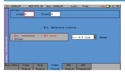
The Video Timing menu displays the relationship between the selected video input with respect to the locking reference input.
