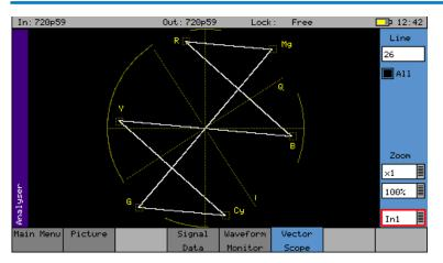
The Vectorscope menu displays the selected input in the form of a vectorscope. This may be set to show either the 100% bar positions or 75% positions. The colour bar position boxes will change according to the colour space for the current input video standard.
