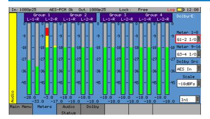
The Audio Meters menu displays up to 16 audio channels. The source for each block of 8 meters may be independently set to allow simultaneous metering of 8 inputs and 8 outputs or all 16 channels in an embedded SDI stream.
