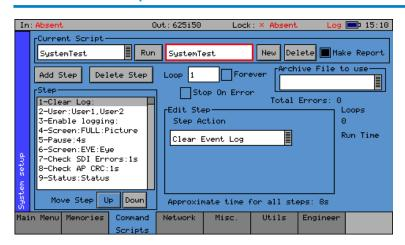
The Command Scripts menu allows the Sx instrument to run predefined scripts.
