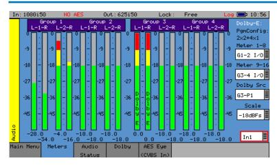
The Audio Meters menu displays up to 16 audio channels. The source for each block of 8 meters may be independently set to allow simultaneous metering of 8 inputs and 8 outputs or all 16 channels in an embedded SDI stream.
