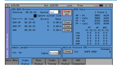
The Video Status menu displays the status of the selected video input and displays any errors that have been found in the data stream.
