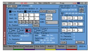
This option provides SMPTE 2022-6 (SDI video over IP) modes for both encapsulation and decapsulation via the dedicated PHABRIX 2022-6 IP 10GE SFP (PHSFP-10SR-2022), and offers SDI-to-IP and IP-to-SDI conversion capability. The SFP can also be managed remotely.
