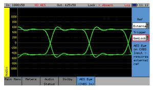
It can be difficult to check that the AES audio signal is correctly locked to the studio reference. The AES Eye option (now as standard) allows the AES waveform to be displayed on the unit. If the studio locking reference is also connected to the unit, then the AES Eye waveform can be displayed locked to this reference.
