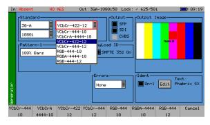
This option (PHSXO-3GADV) provides 3G-SDI Level A and B support including advanced formats: 4:2:2 YUV, 4:4:4 RGB and 4:4:4 YUV at 10/12 bit, and 2K advanced formats including: 4:2:2 YCbCr, 4:4:4 RGB' and 4:4:4 YCbCr at 10/12 bit as well as 4:4:4 XYZ at 12-bit. For broadcast manufacturers this option allows rigorous testing of many more formats beyond the standard signals used in traditional broadcasting.
