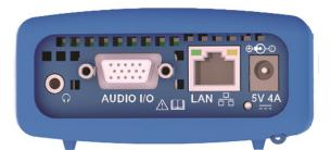
The SxTAG Control panel provide the following connections.
