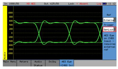
AES Eye menu allows an AES signal of  $75\Omega$ impedance connected to the "PAL/NTSC (AES Eye) In" BNC connector to be displayed as an Eye pattern. This allows the amplitude and quality of the AES waveform to be seen and allows, AES to reference locking, to be checked.
