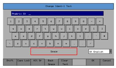
When editing text, the keyboard, left, is displayed to allow easy editing. Move the cursor to select a key to press, and then press 'Ok'. The Shift menu button reveals additional keys available on your current keyboard.
