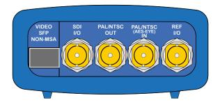
The SxTAG BNC panel provide the following connections.
