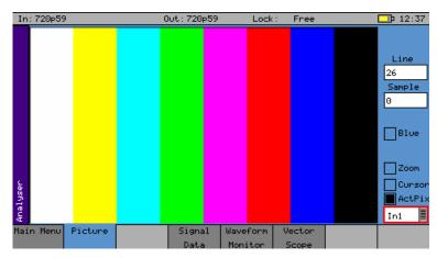
With Picture selected, the video picture is displayed in a window as a down-converted display.
