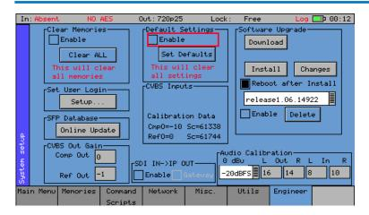
The Engineer menu is used to manage the SxTAG, and among other things allows user access to be setup, and the installation of new versions of software.
