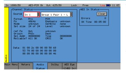
The Audio Status menu shows the Channel Status for the selected audio channel. It is displayed in decoded form as well as a hexadecimal dump of the bytes. The source may either come from the input signal or from the generator for comparison purposes.
