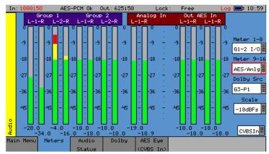
If AES or analogue inputs or outputs are present then these may also be metered. At the bottom of each meter is the current audio level for that channel in dBFs (decibels relative to 0dB full-scale).
