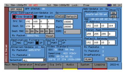
If the SxTAG instrument has the IP 2022-6 Licence option (PHSXO-IP) installed in conjuntion with the PHABRIX IP 2022-6 SFP (PHSFP-10SR-IP), it can transmit or receive 2022-6 IP Flows and convert from SDI-to-IP or IP-to-SDI. See the "System - Engineer" section for details on how to control SDI-to-IP or IPto-SDI Gateway function.
