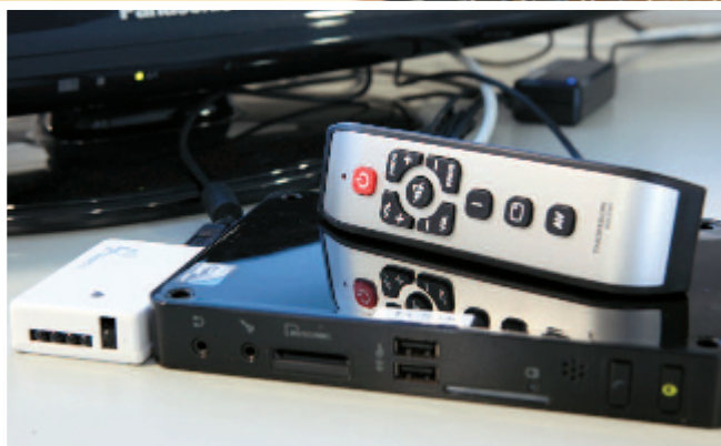
Nettop with remote control from Thomson and IR receiver
